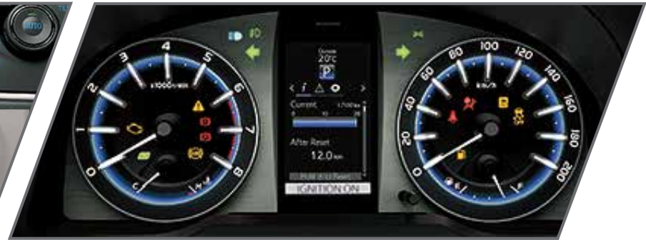
Optitron Meter with 4.2" Colour Multi-information Display*
